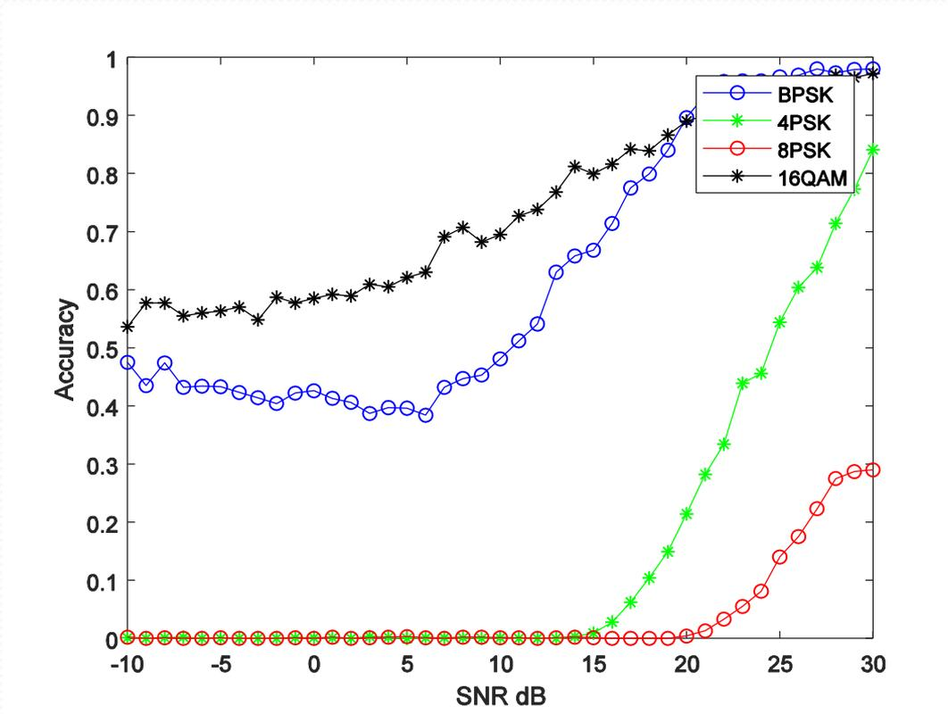
The accuracy for VGG-16 classifier for different modulation types in FBMC with the pilot aided channel estimation over Rayleigh channel.
