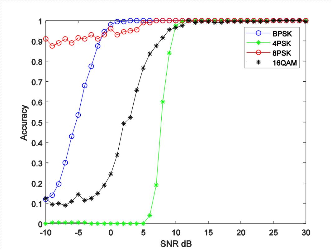
The accuracy for AlexNet classifier for different modulation types in FBMC with the pilot aided channel estimation over AWGN channel.
