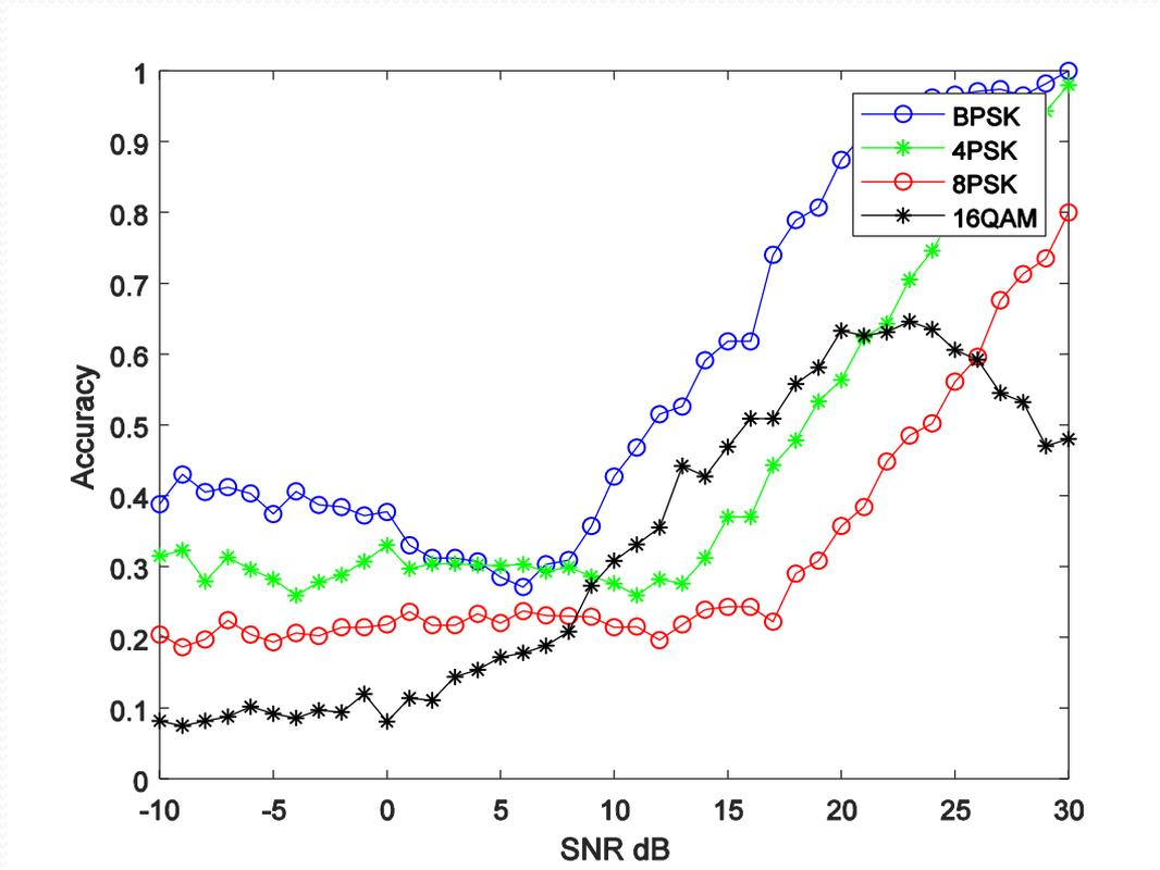
The accuracy for AlexNet classifier for different modulation types in FBMC with the pilot aided channel estimation over Rician channel.
